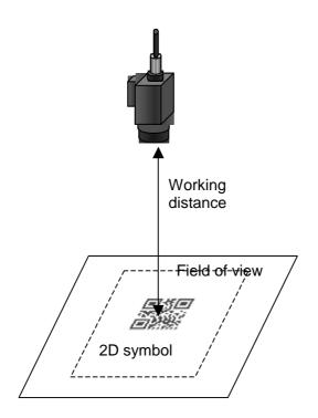
Figure 4-3: Working distance and field of view
