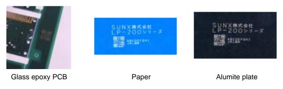
Photo 2-3: Example of CO2 laser marking
