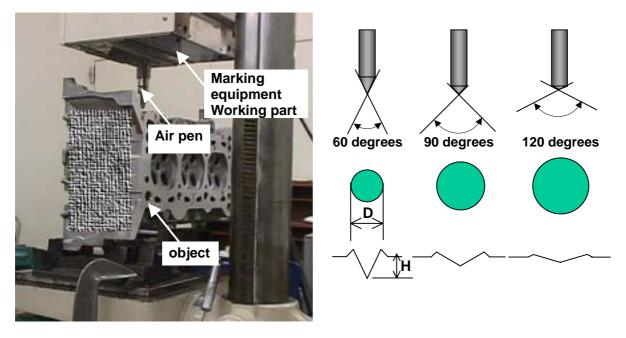
Photo 3-4: Marking test equipment Figure 3-3: Stylus head form and dot appearance
