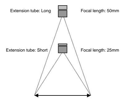
Figure 4-4: Relationship between focal length of lens and extension tube length (Field of view is fixed)
