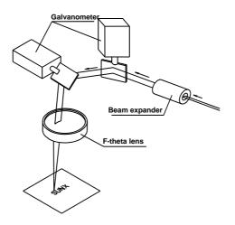
Figure 2-1: Scanning type laser marker
