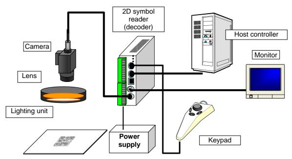
Figure 4-1: Basic setup of 2D symbol reading system
