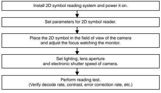
Figure 4-12: Reading test procedures
