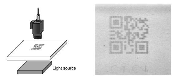
Figure 4-9: Transmitted lighting Figure 4-10: Image captured with transmitted lighting
