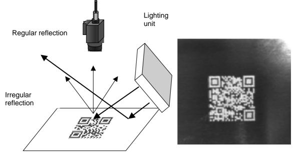
Figure 4-5: Oblique lighting Figure 4-6: Image captured with oblique lighting Oblique lighting is the method, which applies oblique light to the part surface. (See
