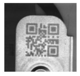
Figure 4-8: Image captured with coaxial lighting
